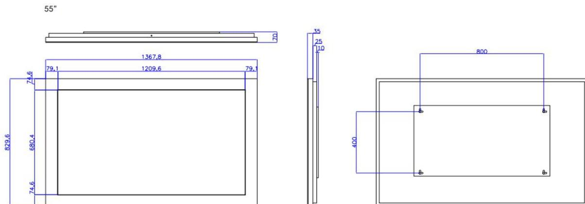
Note: All measurements in millimeters (mm)
