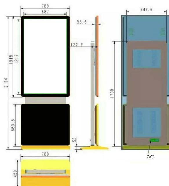
Note: All measurements in millimeters (mm)
