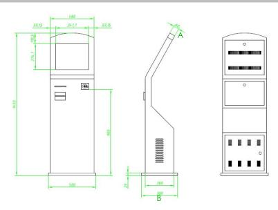
$Note: All\ measurements\ in\ millimeters\ (mm\ {\it --}\ Dimensions\ may\ vary\ depending\ on\ add-on\ peripherals$
